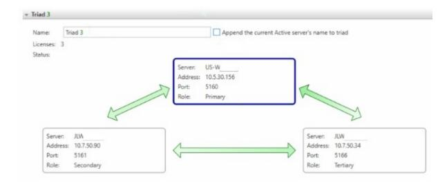
You can manage the triad's settings, such as changing the role of a selected server or replacing a server, by clicking  $\equiv$  to display a menu of management options.
