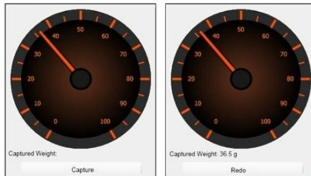
Even though clicking the **Capture** button places a static weight value into a linked data source, the scale display will continue to show a live reading from the scale. This means that the displayed weight value and the value placed into the linked data source
