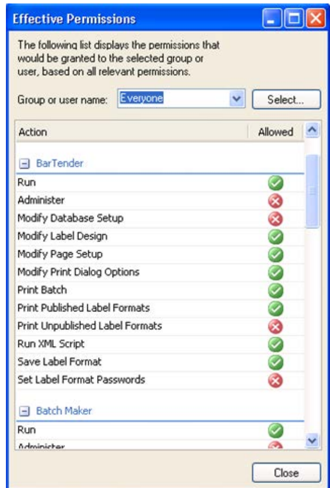
The Effective Permissions view combines a user's individual security settings with the settings from any groups that they may be a member of.
